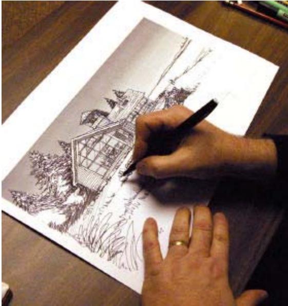
Adding entourage directly onto a print of a SketchUp model.
